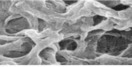
The SEM photograph (above) shows an Electropor chargemodified nylon 6,6 membrane with captured 0.021 micron mono-dispersed latex beads. The combination of Electrokinetic adsorption (positive charge) and mechanical sieving (pore size) provides for enhanced particle removal capability of submicron contaminants like colloidal silica and bacteria fragments.
