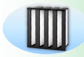
**EARB-V** is designed using the latest State-of-Art technology. Built in a V-shaped construction, it allows EARB-V to increase media area for maximum usage, while sustaining a low initial pressure drop. The unique plastic frame makes the filter light in weight, easy handling during installation.
