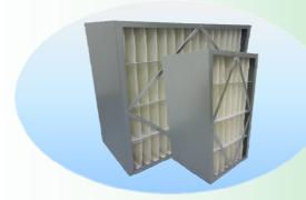
**EARB-DP** is the 1<sup>st</sup> generation of Rigid Box filter created, and the only rigid box type that uses Synthetic media. Using a similar concept as pleat filters, the media is designed in deep pleat with a metal casing, to increase its rigidity. EARB-DP is the best economical choice among rigid box filters, commonly used for Commercial Building applications.
