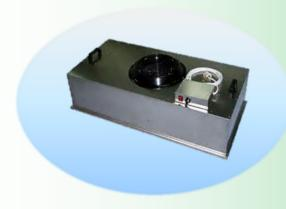
**EAPA-FFU** is commonly used in cleanroom applications, especially for Class 100 and below. It is used extensively in laminar hoods and research centres. It comes with a fan motor in the unit itself with controller, together with a minipleat HEPA at the bottom of the casing.
