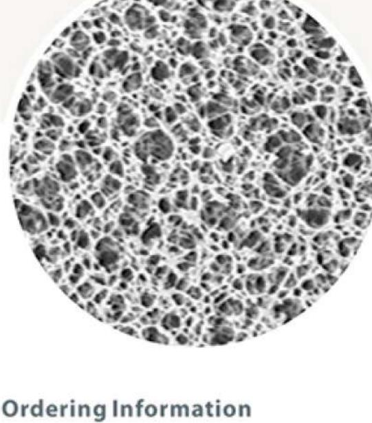
Mixed cellulose ester(MCE) membrane consists of cellulose acetate ester and cellulose nitrate ester. With hydrophilicity, good biological compatibility and low protein binding characteristics, MCE is often used for biological solution filtration, organism analyses and water monitoring.
